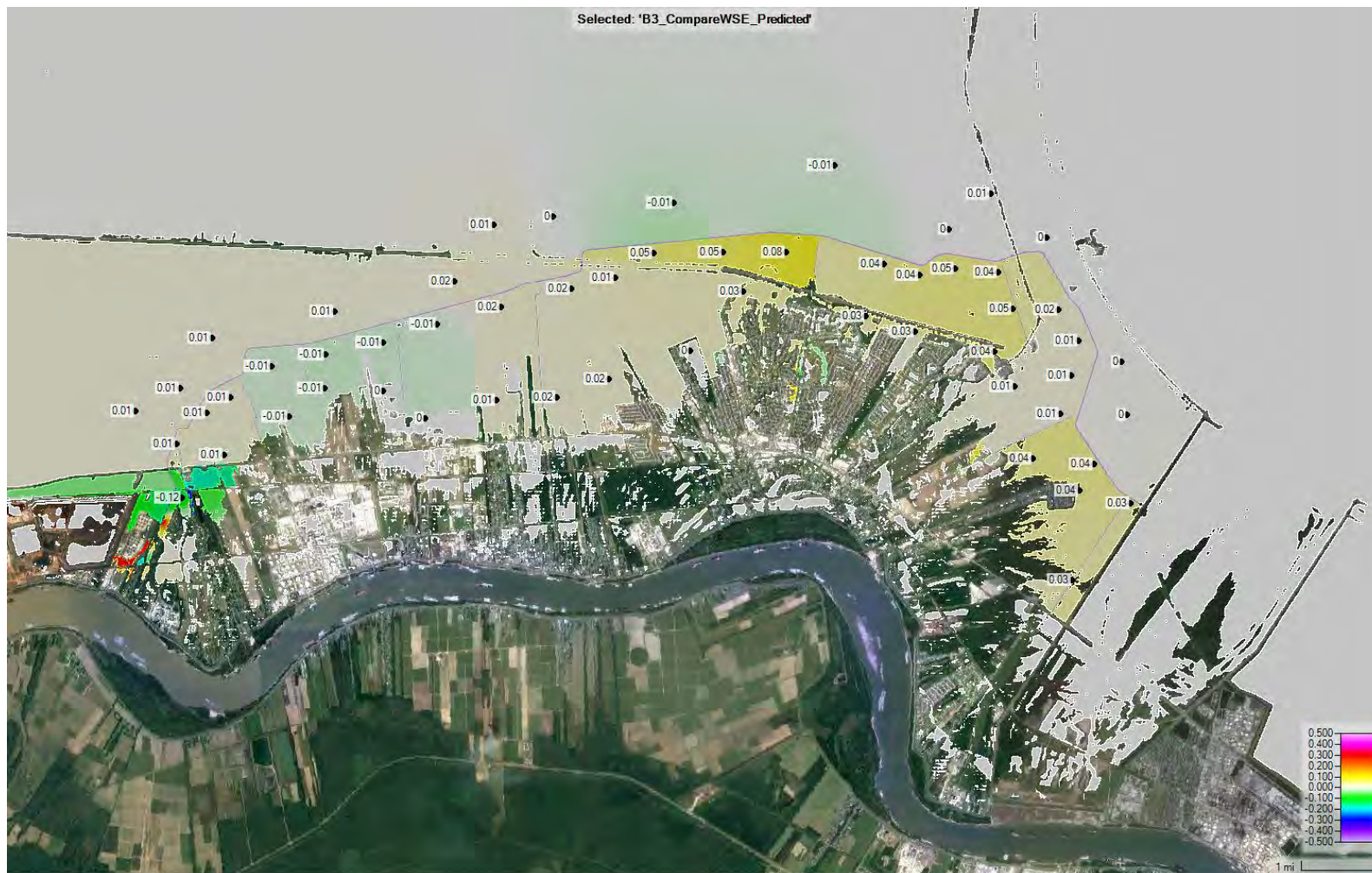
Figure 36 - Maximum water surface elevation difference (with-project minus without-project) for simulation set B3
