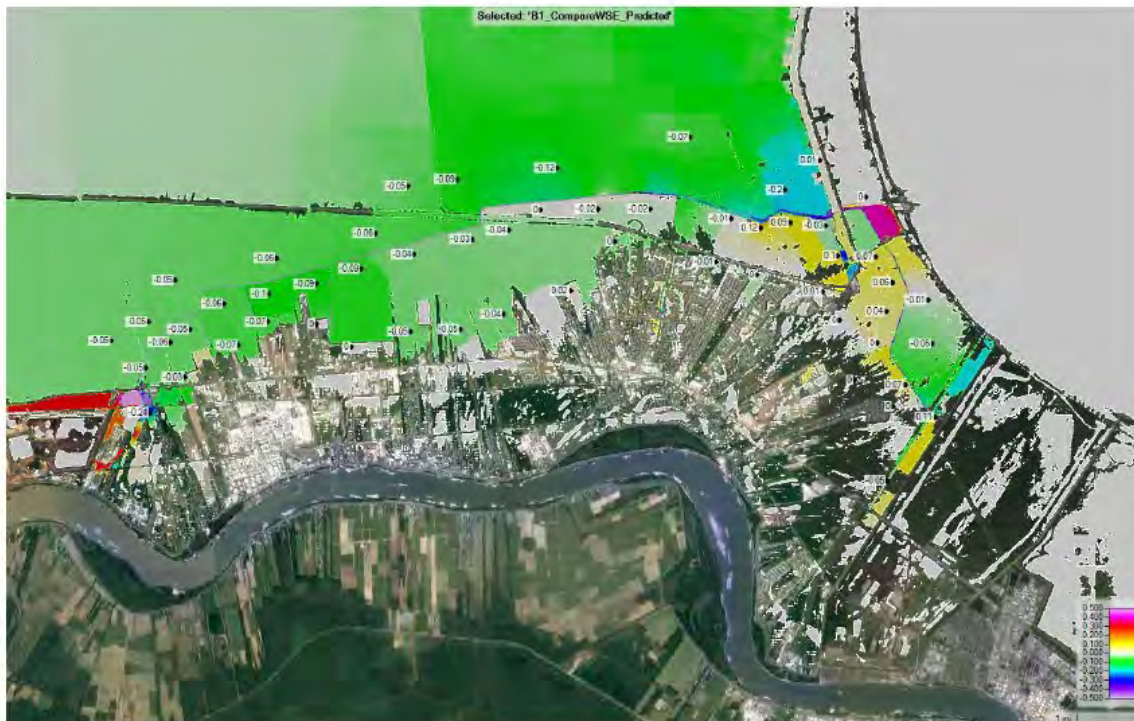
Figure 7. West Shore Lake Pontchartrain results of the additional hydraulic and hydrologic model run to assess for additional indirect impacts associated with changes in the levee system. Figure taken from USACE hydraulic and hydrologic (H&H) model simulations.
