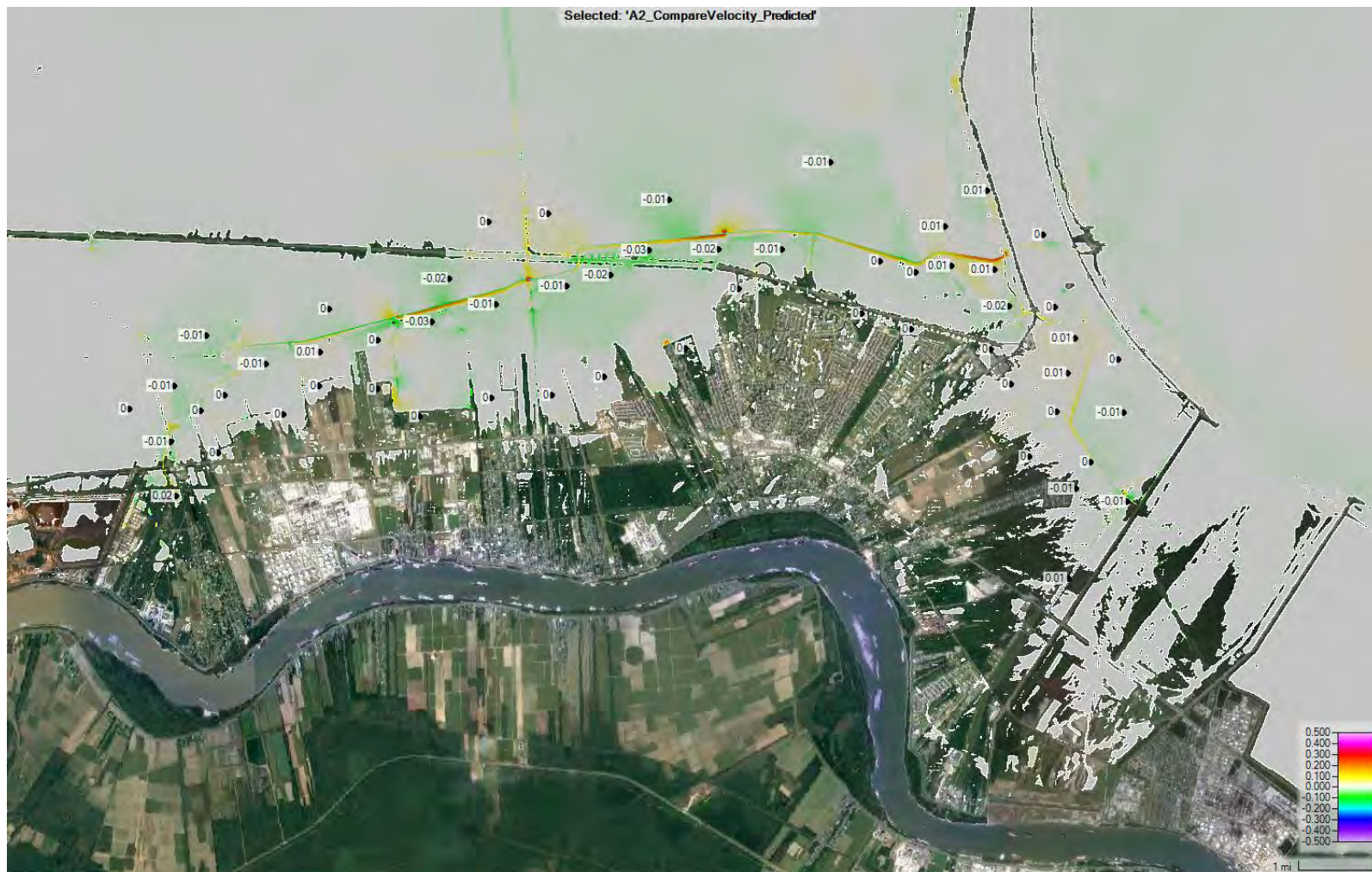
Figure 28 - Maximum water velocity difference (with-project minus without-project) for simulation set A2
