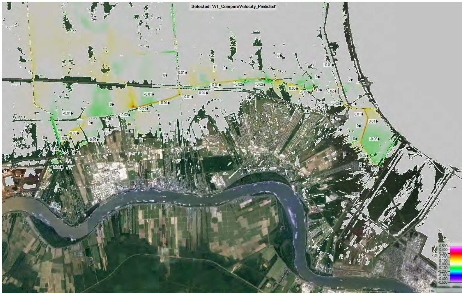
Figure 27 - Maximum water velocity difference (with-project minus without-project) for simulation set A1
