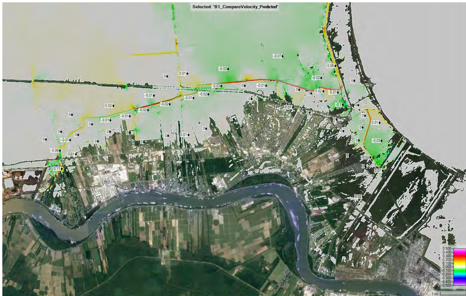
Figure 29 - Maximum water velocity difference (with-project minus without-project) for simulation set B1
