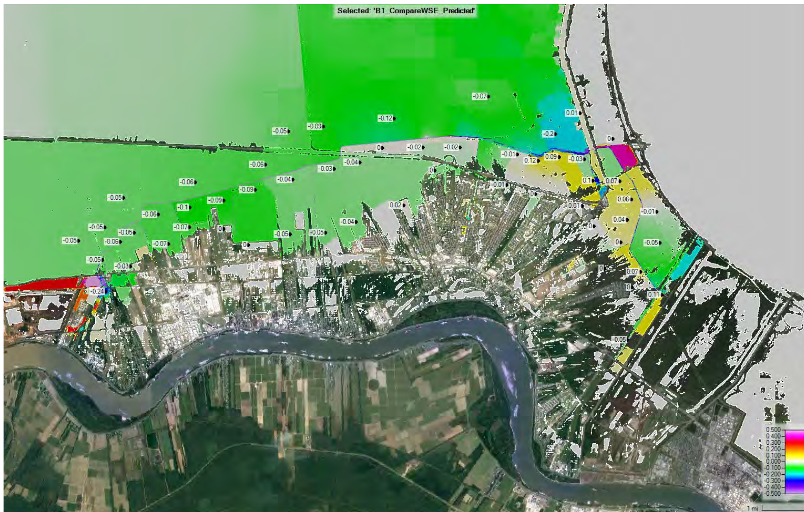
Figure 34 - Maximum water surface elevation difference (with-project minus without-project) for simulation set B1
